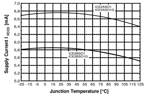
Figure 25 Supply Current  $I_{VCC3}$  vs.  $T_j$
