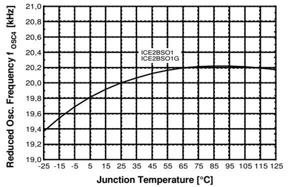
Figure 33 Reduced Osc. Frequency  $f_{OSC4}$  vs.  $T_j$
