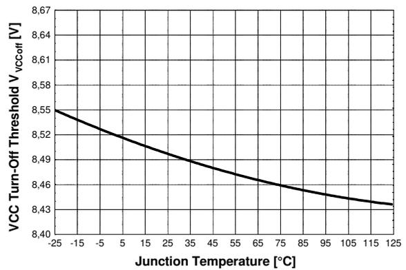
Figure 27 VCC Turn-Off Threshold  $V_{VCCOff}$  vs.  $T_j$
