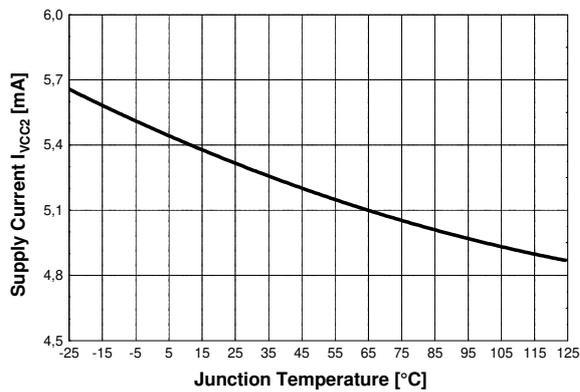
Figure 24 Supply Current  $I_{VCC2}$  vs.  $T_j$
