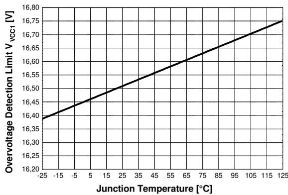
Figure 43 Overvoltage Detection Limit  $V_{VCC1}$  vs.  $T_j$
