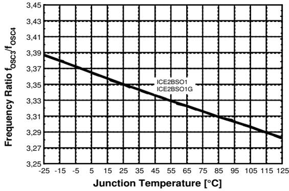
Figure 35 Frequency Ratio  $f_{OSC3} / f_{OSC4}$  vs.  $T_j$
