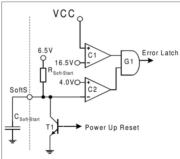
Figure 22 Overvoltage Detection
