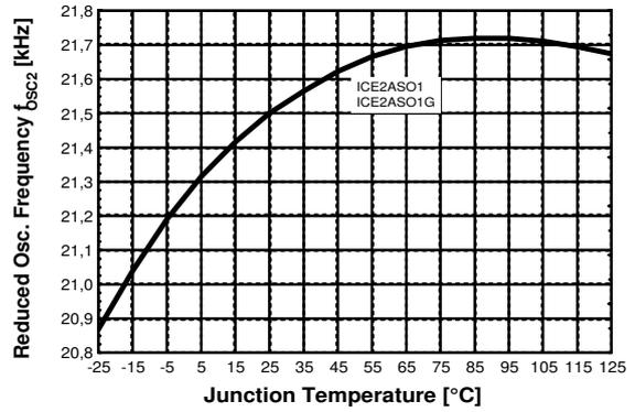
Figure 32 Reduced Osc. Frequency  $f_{OSC2}$  vs.  $T_j$
