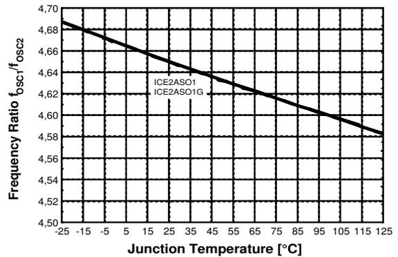
Figure 34 Frequency Ratio  $f_{OSC1} / f_{OSC2}$  vs.  $T_j$
