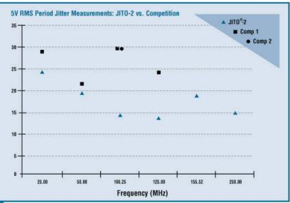
Application Precautions: It is recommended that a sample be evaluated in each application before adding JITO°-2 or any other oscillator to the AVL. This JITO°-2 series of products utilize PLL technology. As a result, overall circuit jitter will often increase if applied to another PLL device. Please contact Fox technical support if you require assistance.
