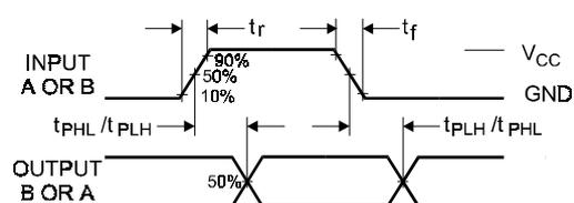
Figure 1. Switching Waveforms
