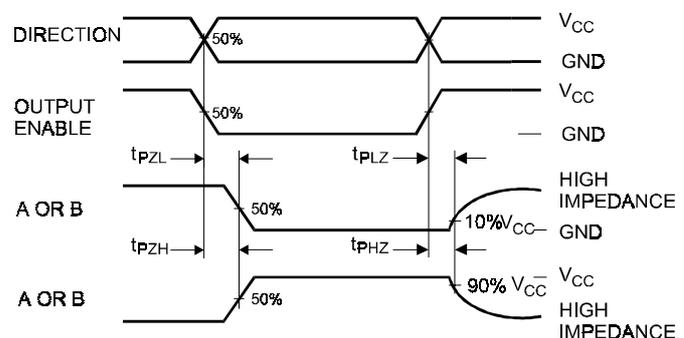
Figure 2. Switching Waveforms
