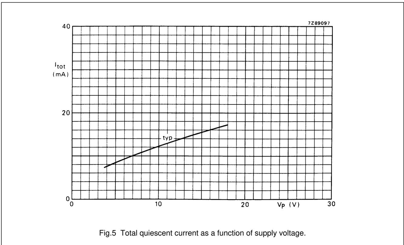
Fig.5 Total quiescent current as a function of supply voltage.
