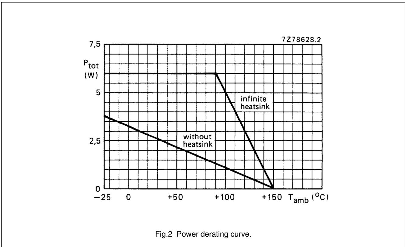
Fig.2 Power derating curve.
