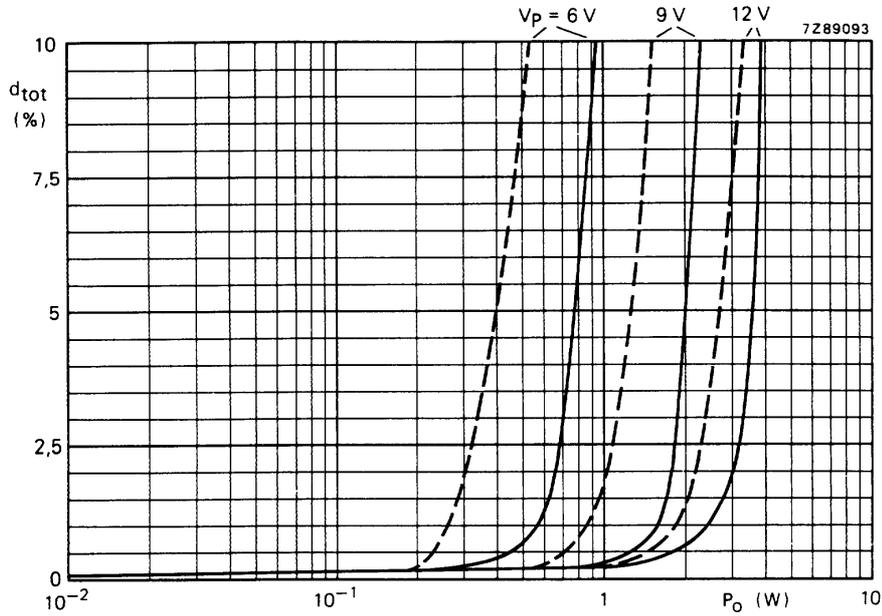
Fig.6 Total harmonic distortion as a function of output power across  $R_L$ ; — with bootstrap; - - - without bootstrap;  $f = 1$  kHz; typical values. The available output power is 5% higher when measured at pin 2 (due to series resistance of C10).
