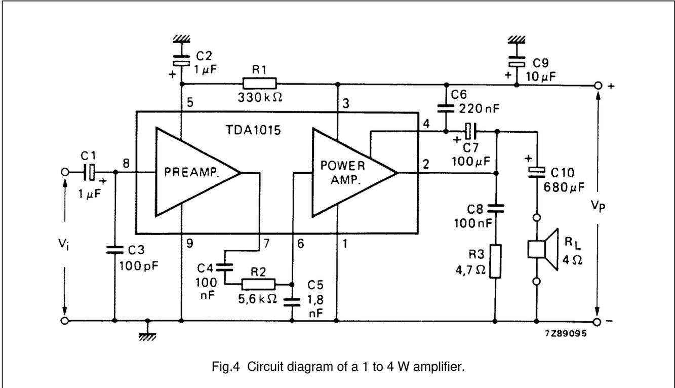
Fig.4 Circuit diagram of a 1 to 4 W amplifier.
