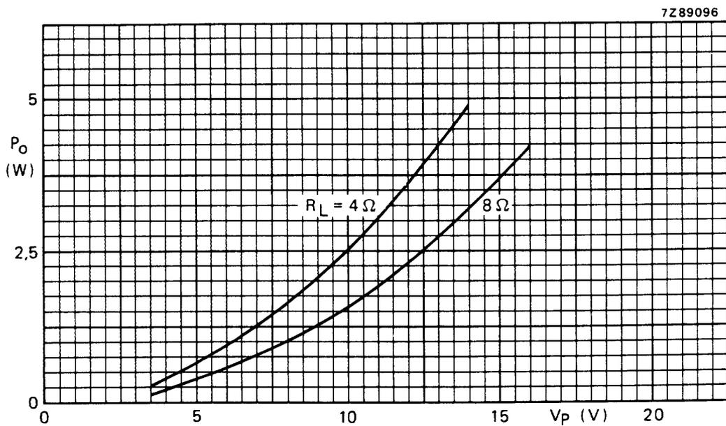
Fig.7 Output power across  $R_L$  as a function of supply voltage with bootstrap;  $d_{tot} = 10\%$ ; typical values. The available output power is 5% higher when measured at pin 2 (due to series resistance of C10).
