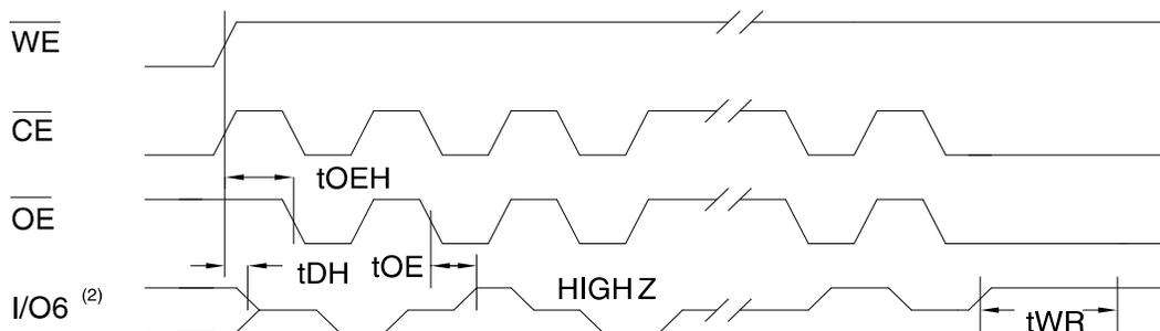
Notes: 1. Toggling either  $\overline{\text{OE}}$  or  $\overline{\text{CE}}$  or both  $\overline{\text{OE}}$  and  $\overline{\text{CE}}$  will operate toggle bit.
