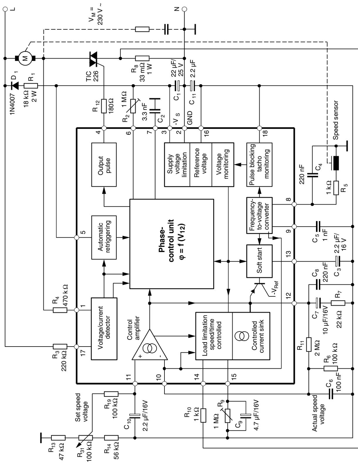
**Figure 10-18.** Speed Control, Automatic Retriggering, Load Switch-off, Soft Start
