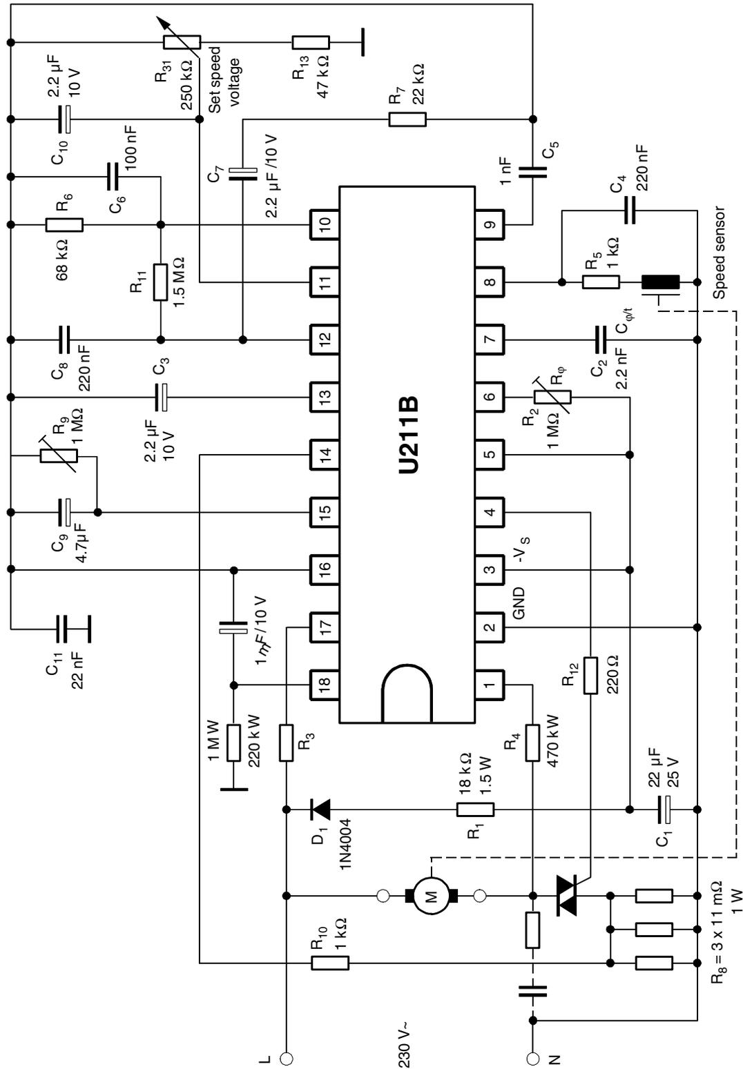
Figure 10-21. Speed Control with Reflective Opto Coupler CNY70 as Emitter
