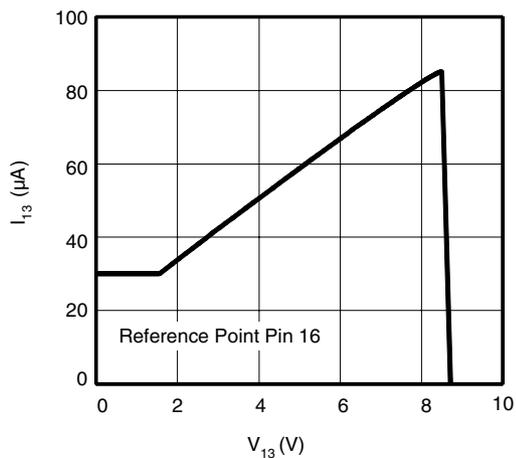
Figure 10-3. Soft-start Charge Current (f/V Converter Active)
