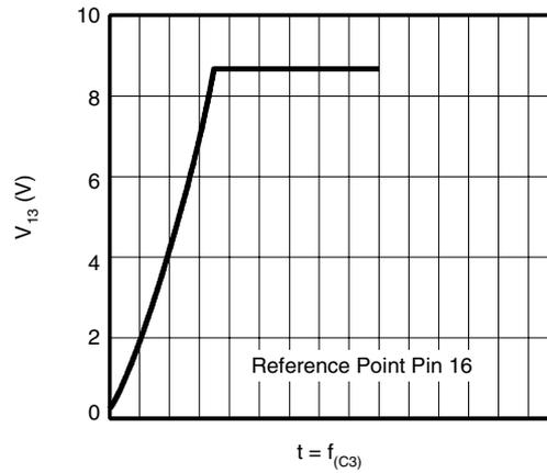
**Figure 10-5. Soft-start Voltage (f/V Converter Active)**
