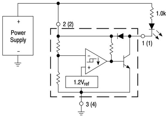
Figure 11. Voltage Monitor
