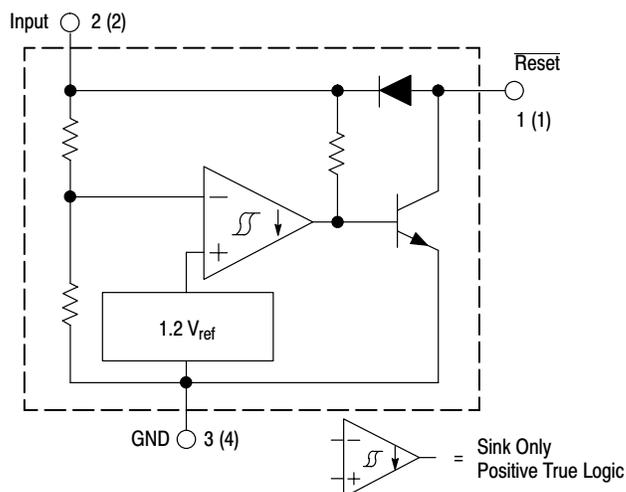
Pin numbers adjacent to terminals are for the 3-pin TO-92 package.
