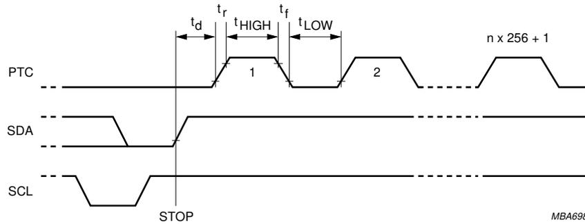
Fig 11. n bytes E/W cycle (n = 2 to 7).
