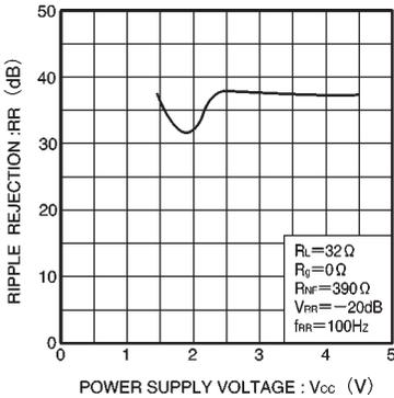
Fig. 11 Ripple rejection ratio vs. power supply voltage
