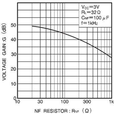
Fig. 13 Voltage gain vs. feedback resistor value
