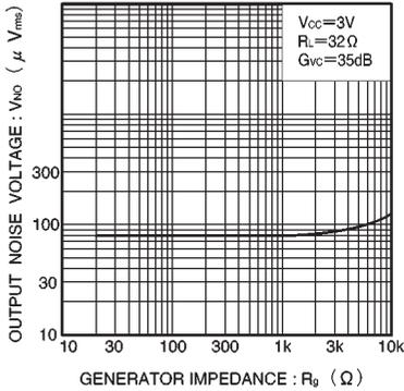
Fig. 9 Output noise voltage vs. signal source impedance
