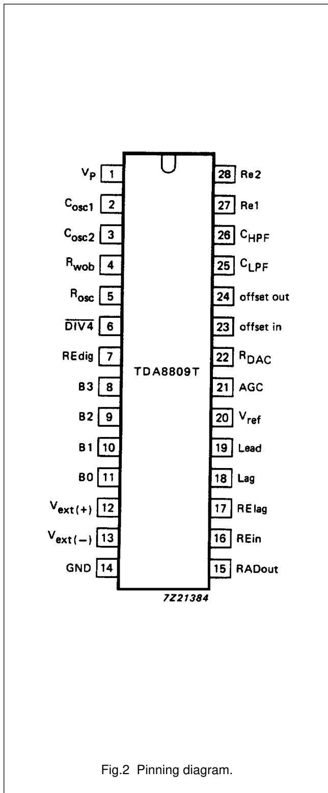
Fig.2 Pinning diagram.
