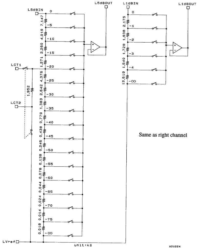
Equivalent Circuit for Fader Volume Section
