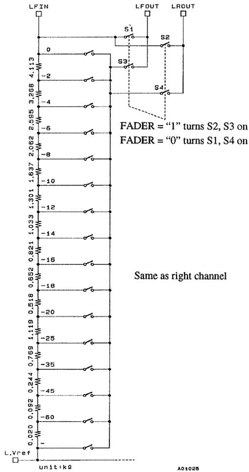
When data of  $-\infty$  is transferred to main volume control 1 dB step, S1 and S2 open and S3, S4 are turned on simultaneously.
