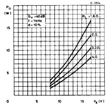
Figure 4. Output power vs. load resistance  $R_L$
