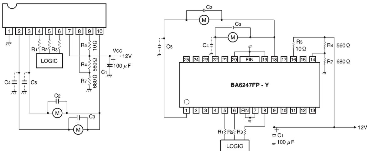
C2, C3: Capacitors for preventing parasitic oscillation. Though the optimum capacitance depends on such PCB arrangement factors as the power supply circuit, motor characteristics, and conductor foil patterns, a range of 0.011 µF is recommended.
