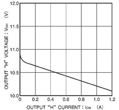
Fig.9 Output high level voltage vs. output current
