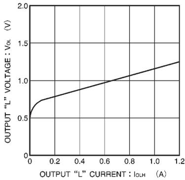
Fig.10 Output low level voltage vs. output current
