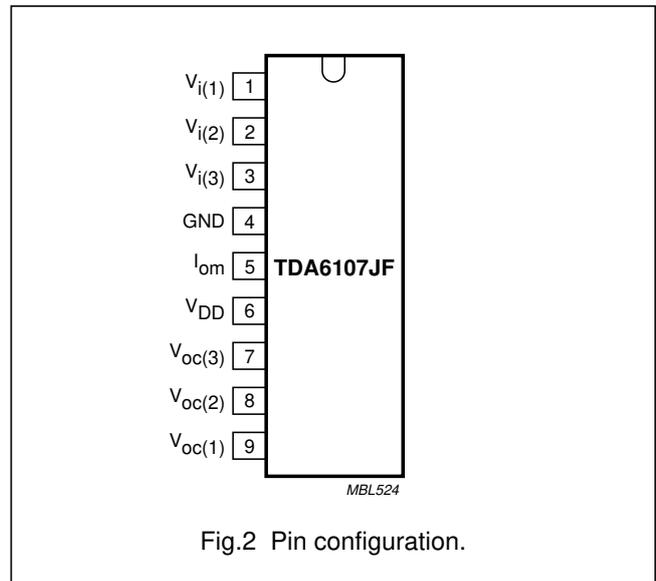
Fig.2 Pin configuration.
