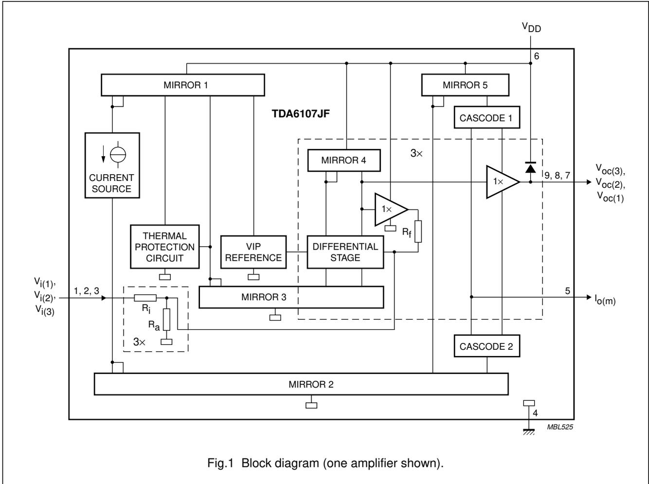
Fig.1 Block diagram (one amplifier shown).
