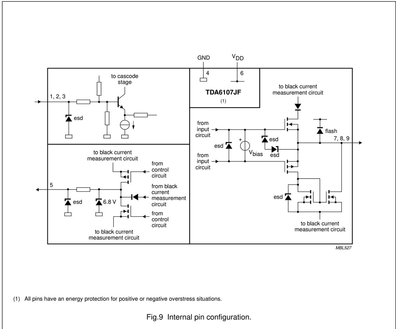
Fig.9 Internal pin configuration.
