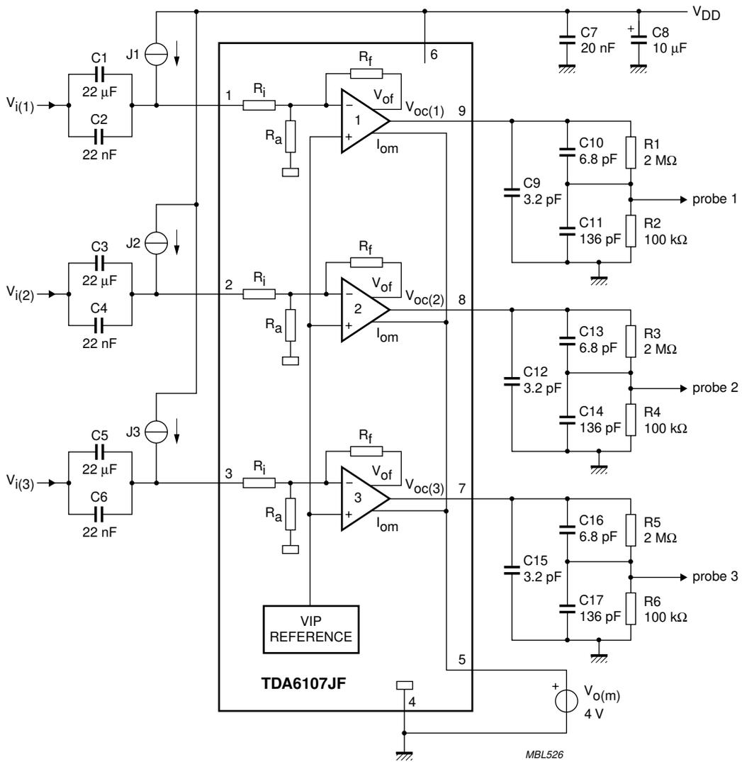
Current sources J1, J2 and J3 are to be tuned so that  $V_{o(c)}$  of pins 9, 8 and 7 is set to 100 V.
