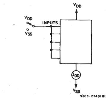
Fig. 10—Quiescent device current test circuit.
