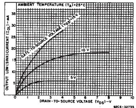
Fig. 3—Minimum n-channel output low (sink) current characteristics.
