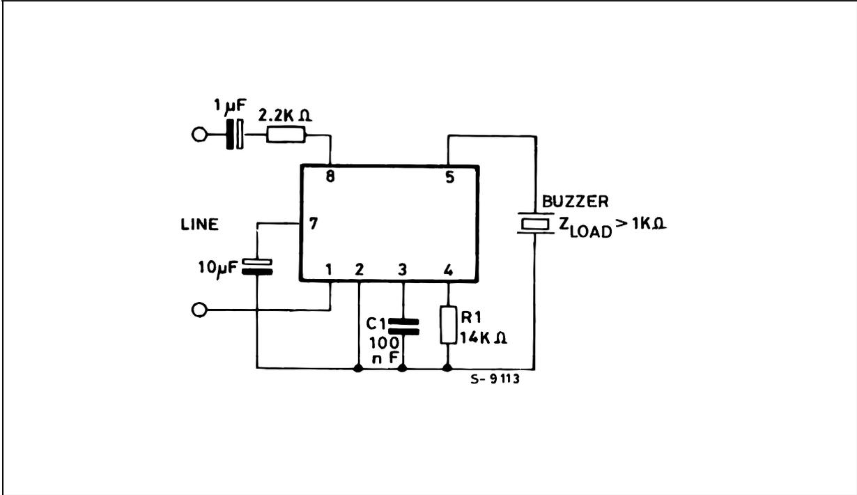
Figure 3 : Typical Application with Loudspeaker (no transformer needed)
