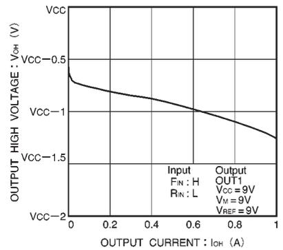
Fig.5 Output high level voltage vs. output current
