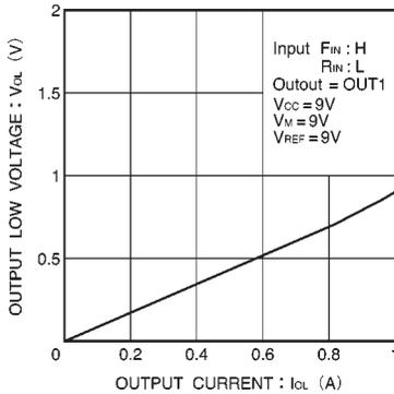
Fig.6 Output low level voltage vs. output current
