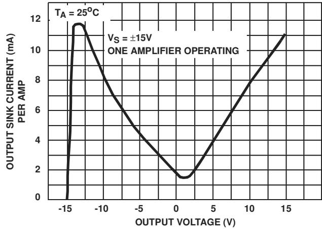
FIGURE 21. OUTPUT SINK CURRENT vs OUTPUT VOLTAGE
