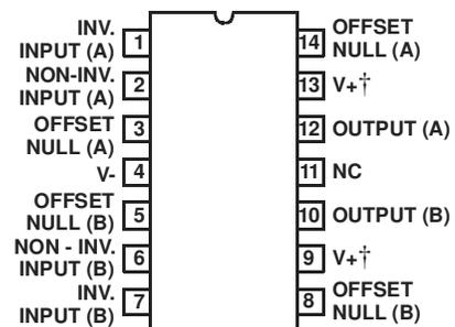
† Pins 9 and 13 internally connected through approximately 3Ω.
