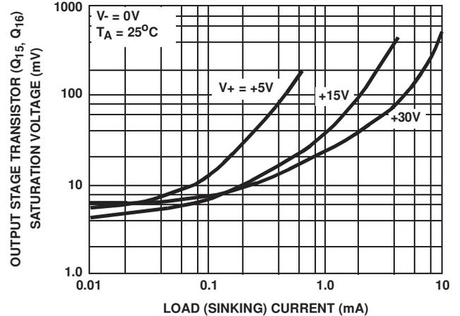
FIGURE 24. VOLTAGE ACROSS OUTPUT TRANSISTORS Q<sub>15</sub> AND Q<sub>16</sub> vs LOAD CURRENT
