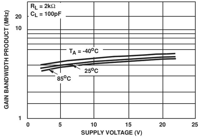
FIGURE 14. GAIN BANDWIDTH PRODUCT vs SUPPLY VOLTAGE
