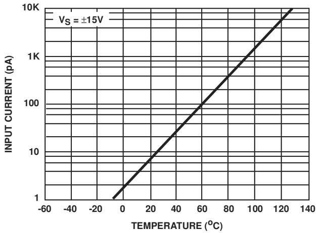
FIGURE 27. INPUT CURRENT vs TEMPERATURE
