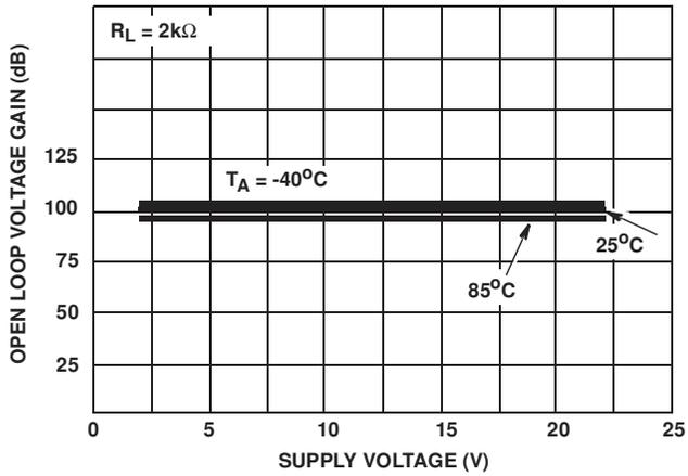
FIGURE 13. OPEN LOOP VOLTAGE GAIN vs SUPPLY VOLTAGE
