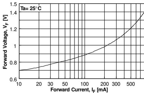
Figure 5. Forward Voltage vs Forward Current
