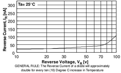
Figure 2. Reverse Current vs Reverse Voltage
