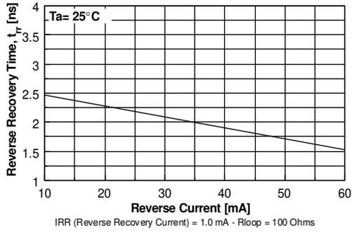
Figure 7. Reverse Recovery Time vs Reverse Current
