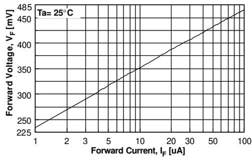
Figure 3. Forward Voltage vs Forward Current
