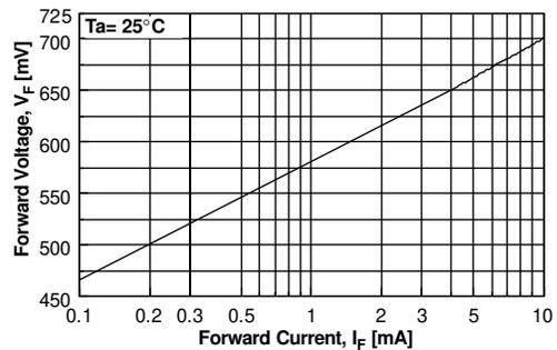
Figure 4. Forward Voltage vs Forward Current
