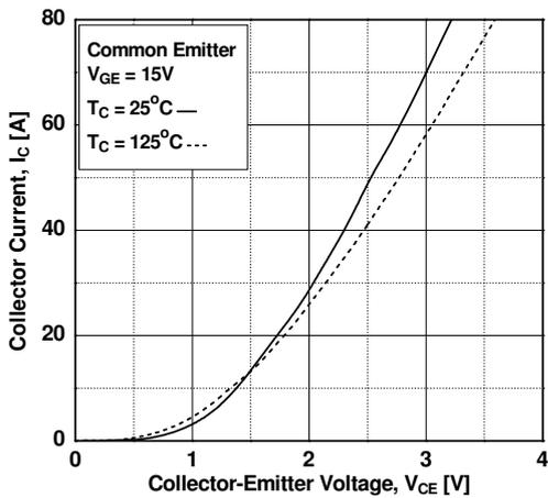
Figure 4. Transfer Characteristics
