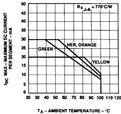
Figure 10. Maximum Allowable DC Current vs. Ambient Temperature.
