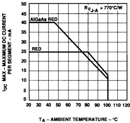
Figure 3. Maximum Allowable DC Current vs. Ambient Temperature.
