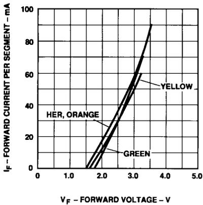
Figure 11. Forward Current vs. Forward Voltage Characteristics.
