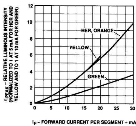
Figure 12. Relative Luminous Intensity vs. DC Forward Current.
