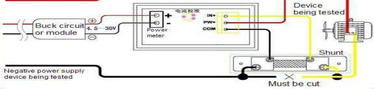
**Nonisolated - Outside power supply - wiring diagram**
