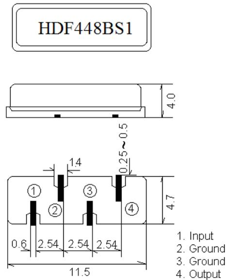
■ Recommended layout of PCB(MM) (Tolerance  $\pm 0.2$ MM)
