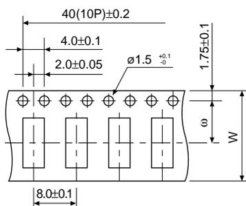
SSP-T5/T6 (Conforms with IEC60286-3)
