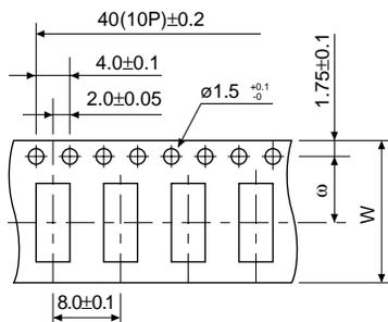
HTF-VT/VTC (Conforms with IEC60286-3)
